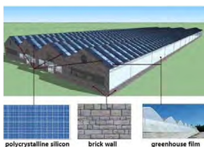
Figure 18: The megawatt photovoltaic power station on the roof of greenhouse
