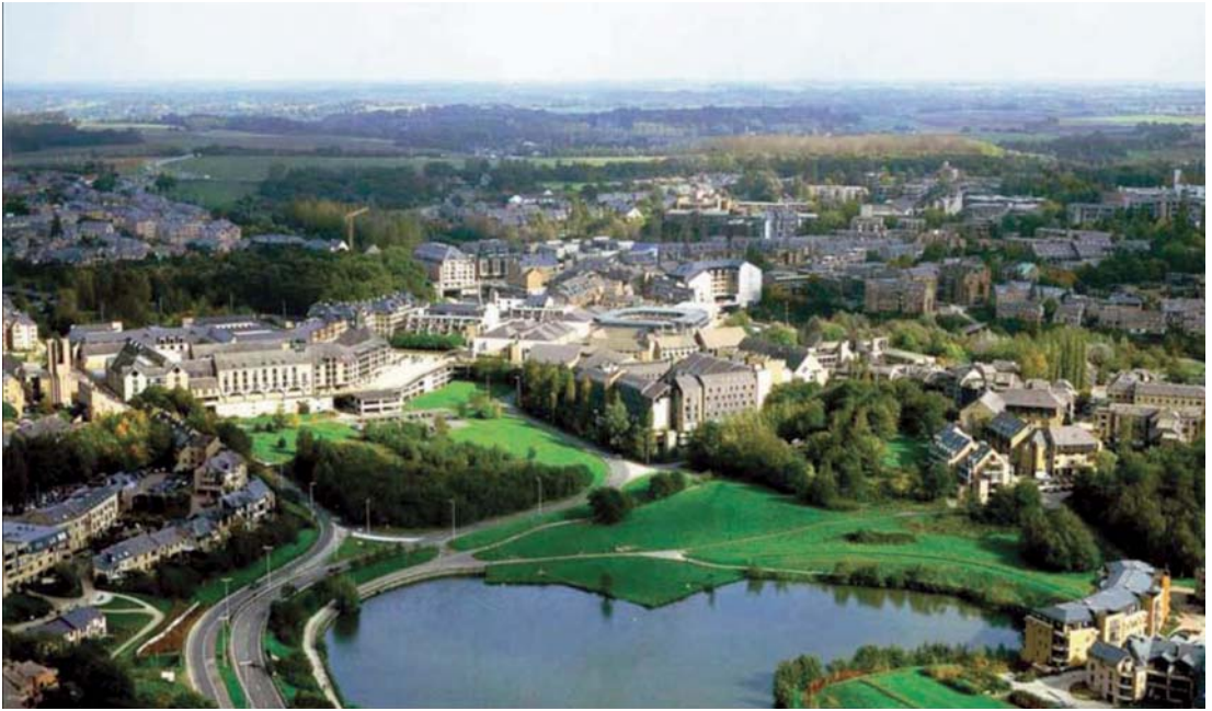
Figure 16: The university town of Louvain-la-Neuve (New Louvain) is a prime example of a sustainable, liveable development. It is centred on a new railway station and is entirely pedestrian, parking space being provided outside the town or underground. It has many ecological features and has a present population of 40.000. All storm water is led to a reservoir landscaped as an artificial lake, with a stable water level Source: Wilhelm & Co.
