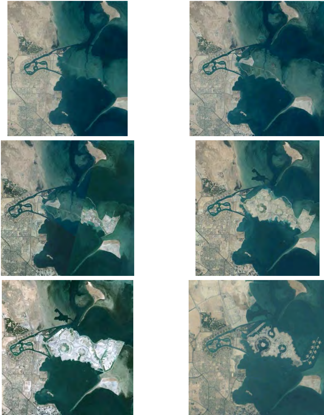
Figure 5. Reclamation Work for The Pearl: October 2003 (Top-Left), August 2004, January 2005, November 2005, April 2006, January 2007 (Bottom-Right).
