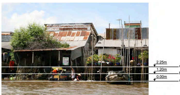
Figure 3: Different river water levels in Can Tho river with (a) normal level in dry season on 4th May 2013; (b) low level in flooding season on 22nd November 2013; and (c) highest level in flooding season on 8th November 2013 (source: Author).
