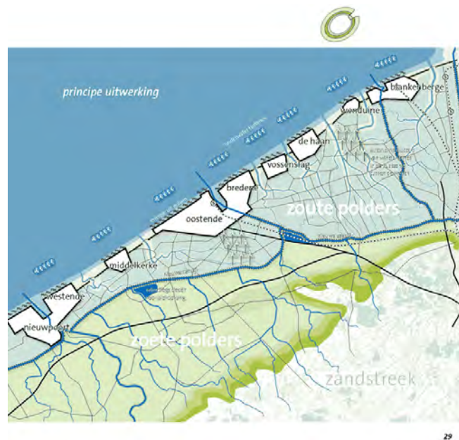
Figure 9: Coastal water park, with saline land (light blue), and freshwater land (light green). Settlement areas are white with a black outline symbolising dikes. (Royal Haskoning 2012)
