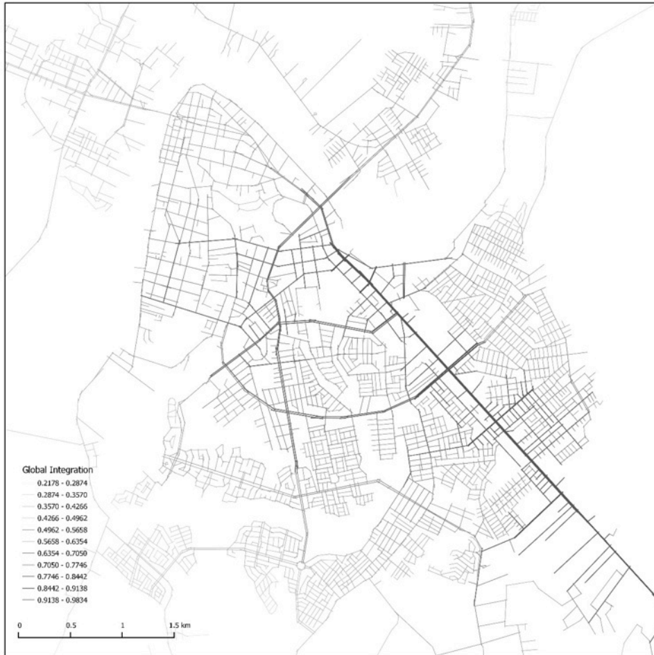
Figure 2: Valdivia current situation. Integration map with radius n , integration of lines shown from dark to light.
