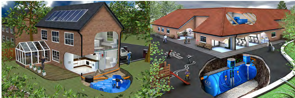
Fig. 4.2.13. Rainwater harvesting for domestic use (left) and for industry (right)
