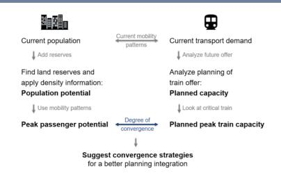
The analysis is directly done for the critical moment in the system, which is in the corridor under investigation the train in the morning peak hour (peak train).
