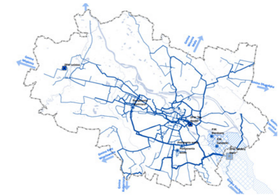
Figure 9 Water supply: existing network
