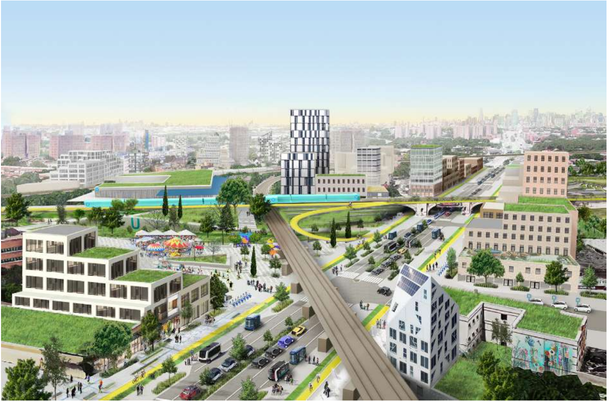
Figure 4: Trees, green roofs, and other vegetation can help cool urban communities by deflecting radiation from the sun and releasing moisture into the atmosphere (Credit: Only If + One Architecture for RPA)
