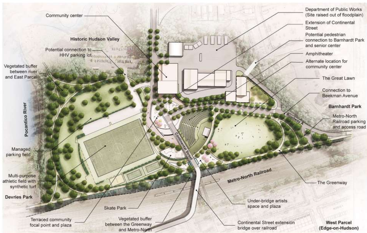
Figure 4: Concept Site Plan for the East Parcel Redevelopment, Sleepy Hollow, NY (Source - WSP USA)
