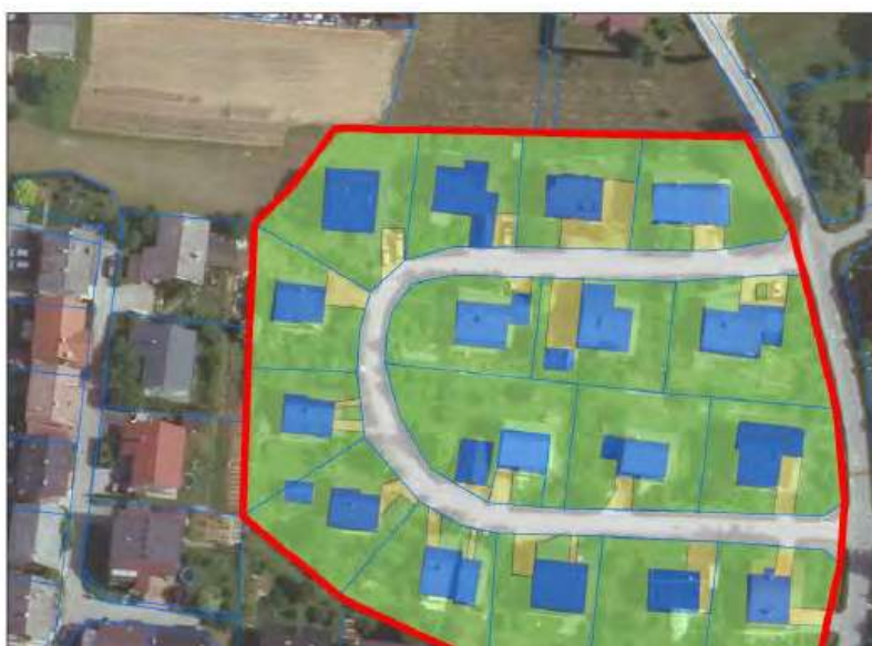
Figure 1 An example from the Arc-GIS database showing the analysed morphological unit for the case of family-housing typology (red – boundary of studied morphological unit, blue – buildings, yellow and grey - private and public traffic surfaces, green – private gardens).
