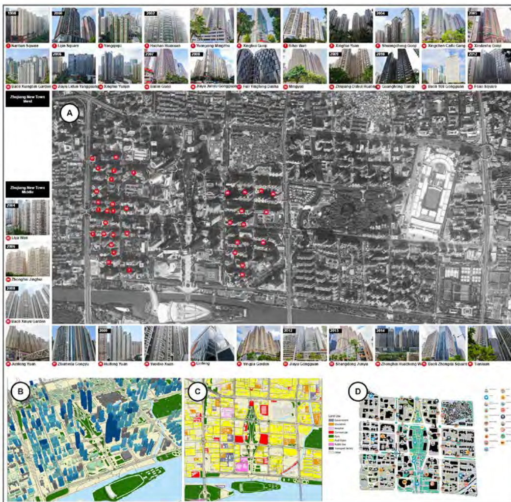
Figure 6. ZJNT. A: Aerial photo with building types ordered by constructed year; B: 3D building volume model coloured by FAR; C: Land use; D: Main features and facilities. Source: author.
