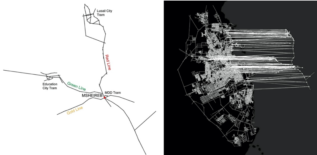
Figure 14: Demonstration of (right) close-up view of the modeling indicating key identifying rail lines and locations, and (left) linking methodology for incorporating the public rail/tram networks before computer processing of configurational measures in the space syntax model of Metropolitan Doha in 2020 (Source: QUCG-CENG-20/21-1).
