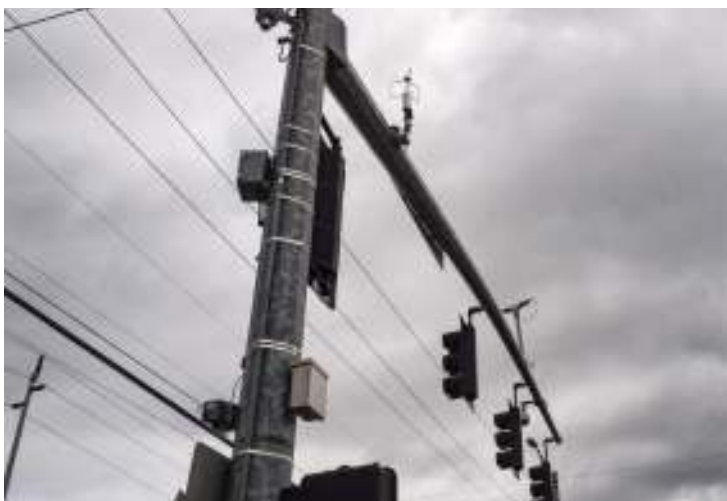
Figure 10: The traffic signal pole and mast arm equipped with a 3D sonic anemometer for wind speed and direction, temperature and relative humidity probe, and cameras and radar for traffic counts on the SW corner of the intersection of SE 122nd Ave and SE Division St.
