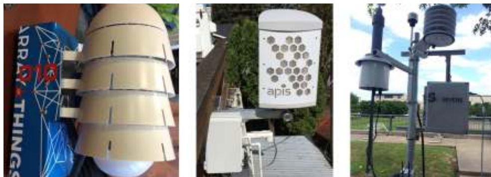
Figure 8: Images of the three climate and air quality sensor devices to be deployed in the City of Portland. From left to right, Argonne National Laboratory/University of Chicago's Array of Things node, Apis SensorCell node, SenSevere RAMP device
