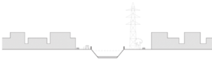
3. The sub-drain is channelled, increasing water velocity and disrupting ecosystems.
