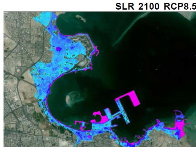
Figure 2 :figure showing the vulnerable areas from Sea Level Rise (SLR)/ Projected coastal flooding of Doha area by 2100
