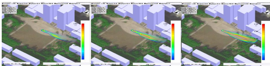
Figure 8. The result of relative concentration, high, medium and low respectively show at breathing height 1.25 m (the lawn space in front of Guanghua Building, Fudan University) Source: the author by Windperfect.
