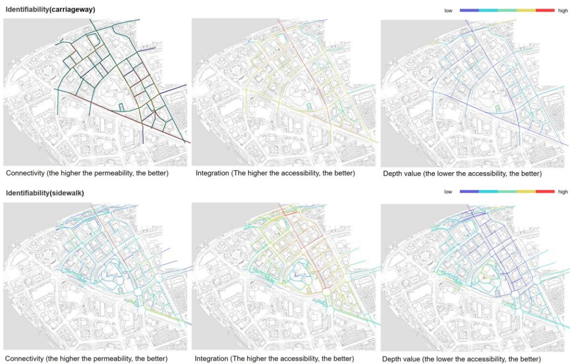
Figure 5. Analysis of street space identification. Source: Author.
