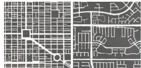
3.2.1.2 These two maps depict, with the same scale, one square mile of two very different street designs. On the left is Philadelphia (PA) with a highly connected street network and on the right Irvine (CA) as an example of lower connectivity, bigger urban blocks, winding streets and many cul-de-sacs.
