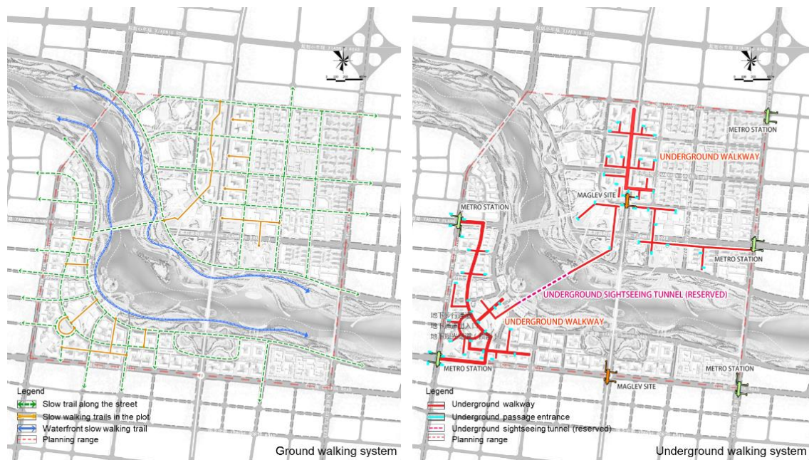
Figure 21. Planning drawing of ground and underground pedestrian system. Source: 'Five Centers Conceptual Urban Design'.
