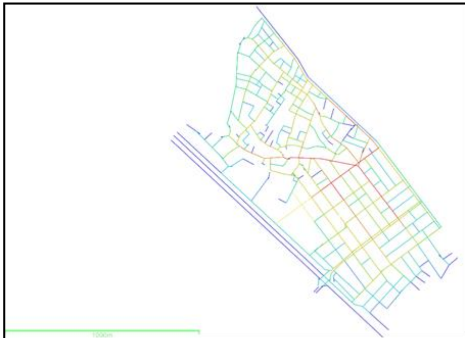
Figure 6. Potential Usage Density of Transportation Axes as a result of Space Syntax Analysis
