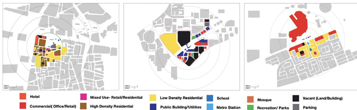
Figure 6: Pedestrian shed radii and 250m, 400m, 600m, and 800m and ground-level land use survey for all urban blocks within 250m of station entrances for (left) Hamad Hospital Station, (center) West Bay Station, and (right) Al Aziziah Station (Image: Authors).
