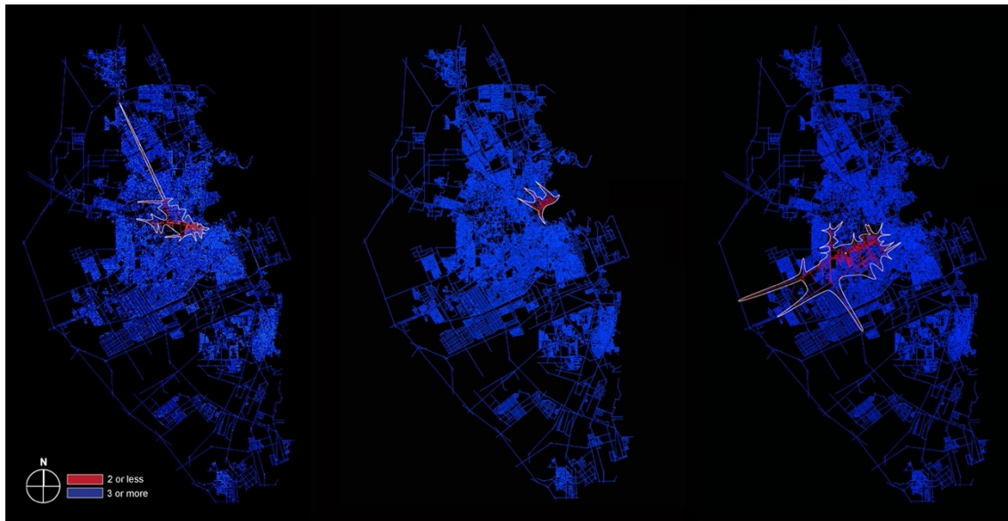
Figure 9: Catchment contour map of all routes within 2 changes of directions or less from the routes on which there are entry/exit points for (left) Hamad Hospital, (center) West Bay QIC, and (left) Al Aziziah metro stations within the spatial network of Metropolitan Doha in 2020 (Image: Authors).
