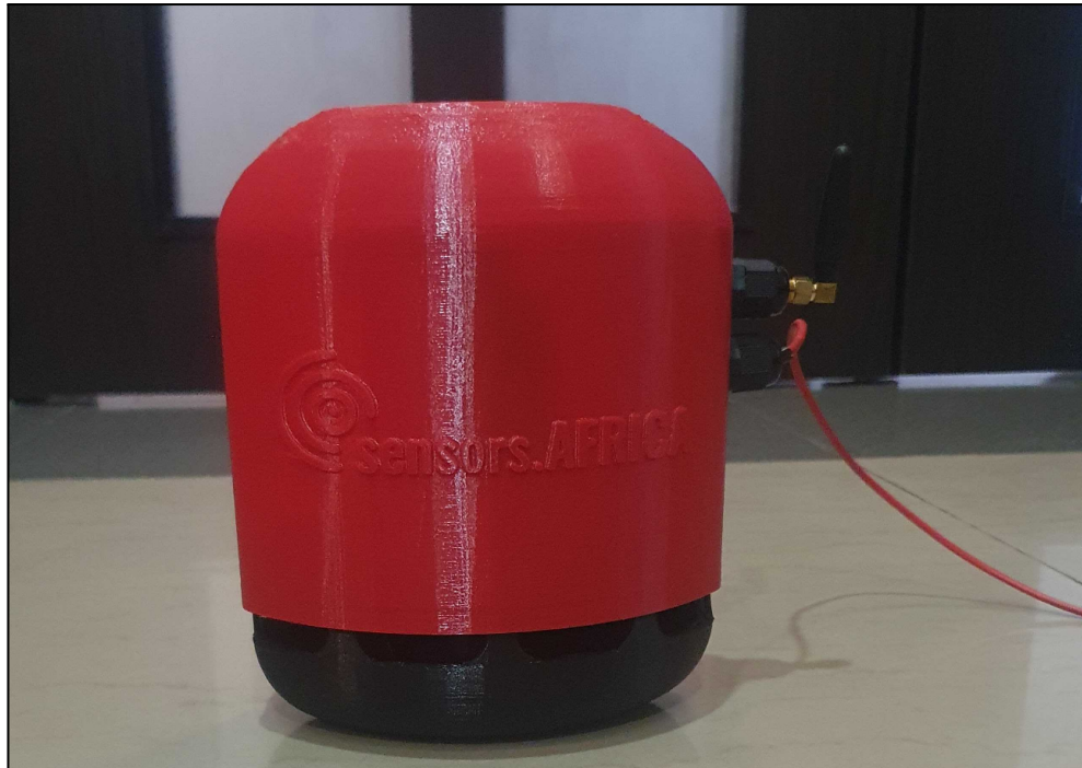
Sensors.AFRICA locally developed outdoor Air Quality monitor
