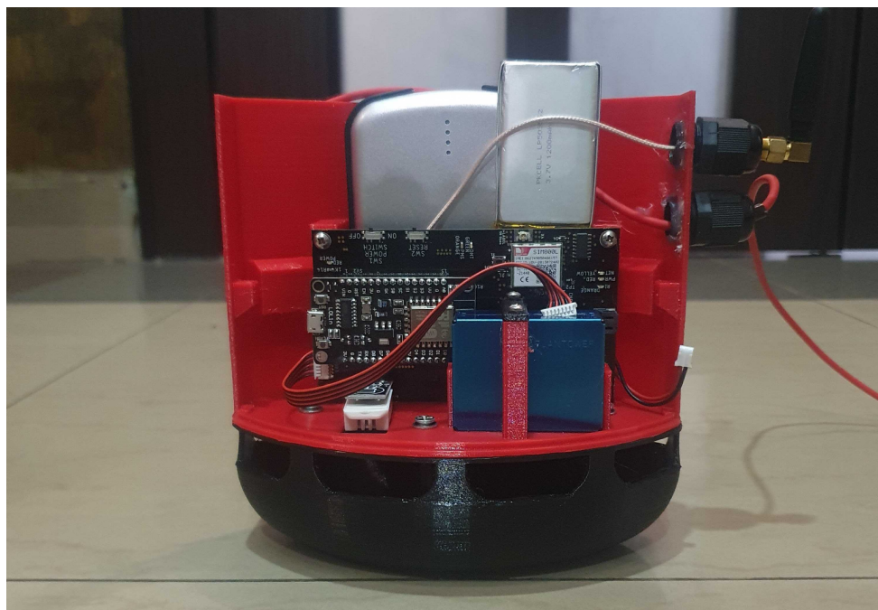
Sensors.AFRICA locally developed outdoor Air Quality monitor
