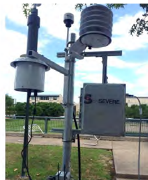
Figure 8: Images of the three climate and air quality sensor devices to be deployed in the City of Portland. From left to right, Argonne National Laboratory/ University of Chicago's Array of Things node, Apis SensorCell node, SenSevere RAMP device
